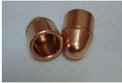
Fig 4.1: Photograph of Class 2 Copper Chromium electrode.
