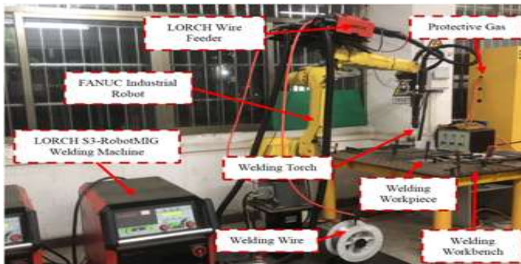
Figure 1: Robotic MIG welding experimental setup and main instrument(Yao et al. , 2025)
